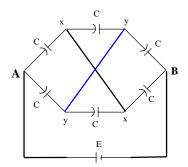
Note: Blue wire is not cutting any other wire as it is on a different plane.
