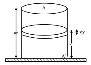
Let's say at any time t the height of water is y and the speed is v. In time dt the height changes by dy and the volume change is dV.
