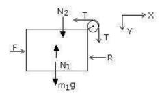
Note:  $m_3$  presses on  $m_1$  by force R (action-reaction). Similarly  $m_2$  presses on  $m_1$  by force  $N_2$  (action-reaction).  $N_1$  is normal force applied on  $m_1$  by the table (or surface).
