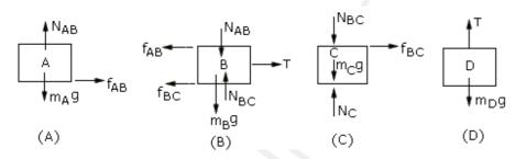
Note (i)  $f_{AB}$  is friction between blocks A and B, and  $f_{BC}$  is friction between blocks B and C. Block B tends to slide towards right with respect to A and C. Hence,  $f_{AB}$  and  $f_{BC}$  act to left on B. As reaction,  $f_{AB}$  and  $f_{BC}$  act to right on A and C respectively.
