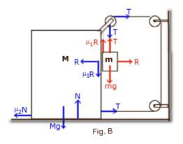
Look at Fig. B indicating the forces - the blue colored are the forces on block M and the orange ones act on block m.
