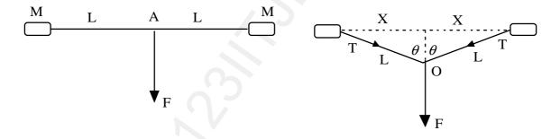
T = Ma (vertical force due to gravity has not been considered as the table is in the horizontal plane)
