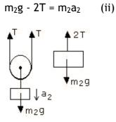
Where  $a_2$  is vertical acceleration of mass  $m_2$ . Note that upward tension on  $m_2$  is 2T applied by both sides of the string.
