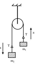
Velocity of masses can be obtained by the following relation obtained from mechanical energy conservation:
