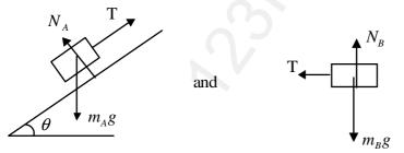
Note that  $m_A g$ , should better be resolved along and perpendicular to the plane, as the block A is moving along the plane.
