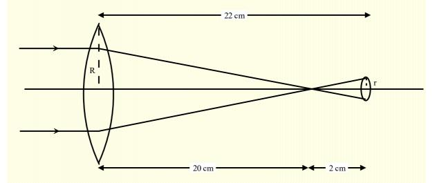
Incident power on the lens = Intensity  $\times$  Cross-sectional area of lens =  $I.\pi R^2$
